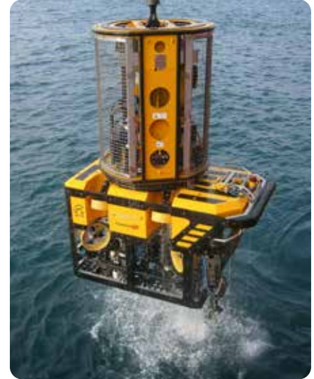
Workclass ROVs allow underwater inspection from vessels
