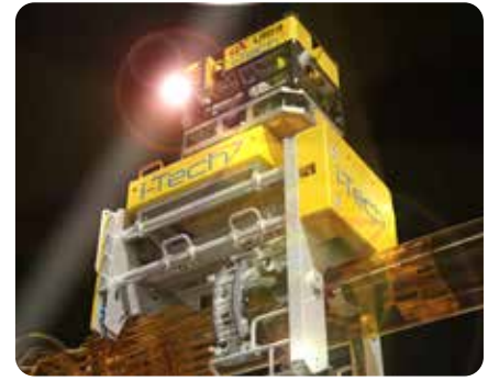
ROV deploying Flange Bolting Tool
